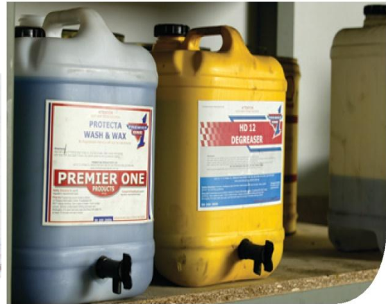
Avoid loss of raw materials and reduce emissions by fitting taps and keeping lids on containers.
