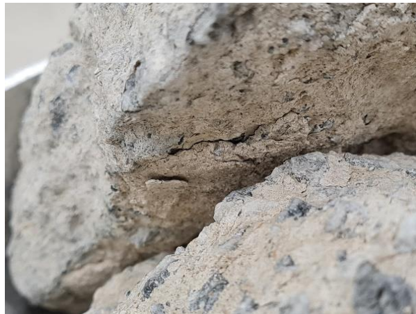
Figure 53. Presence of laminations on the waste surface after 31 days of immersion (3cycles).
