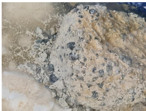
Figure 54. Desegregation during immersion.
