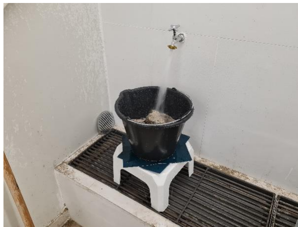
Figure 34. Saturation of the samples.
