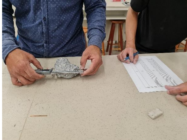
Figure 29. Rock sample shape index obtention.
