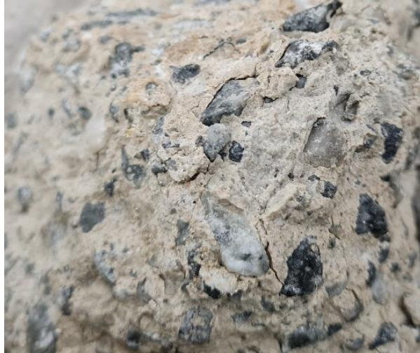
Figure 52. Presence of desegregation on the waste surface after 31 days of immersion (3cycles).
