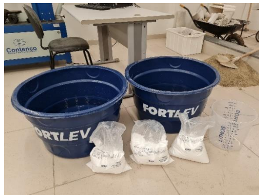
Figure 32. Sodium sulfate and containers used in the laboratory test.
