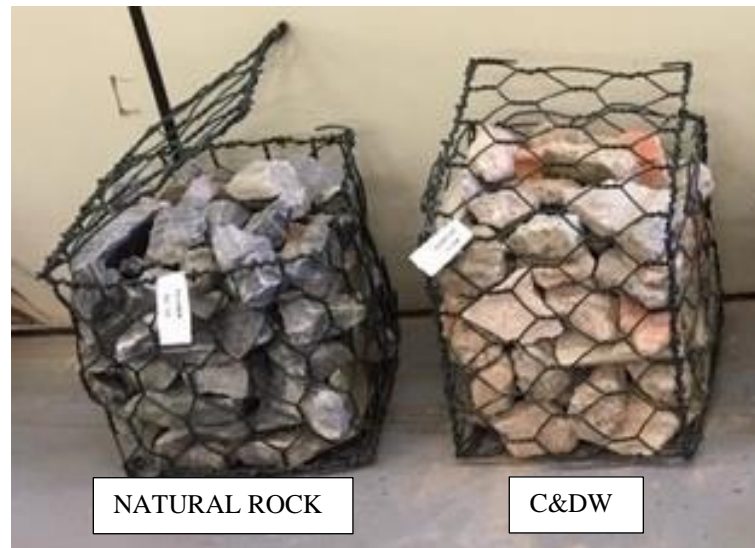
Figure 9. The aesthetic aspect of the C&DW and natural rock.
