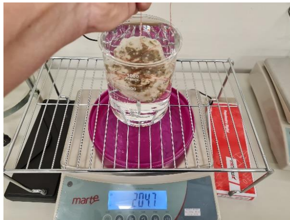
Figure 28. Bulk determination (C&DW and rock coarse soil samples).
