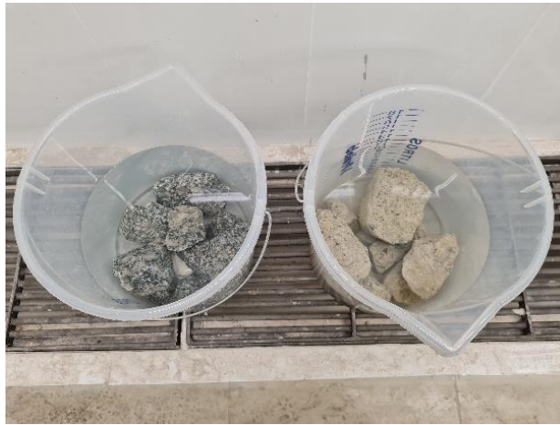
Figure 34. Saturation of the samples.
