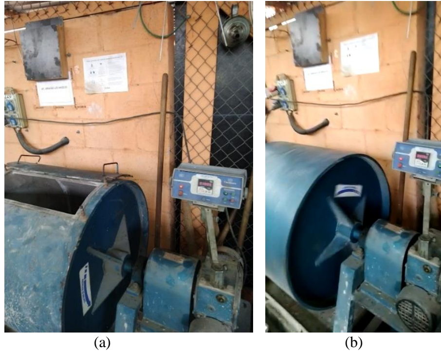
Figure 31. Los Angeles abrasion test being performed
