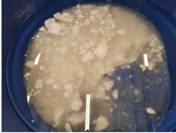
Figure 49. Natural stone container with sodium sulfate solution.
