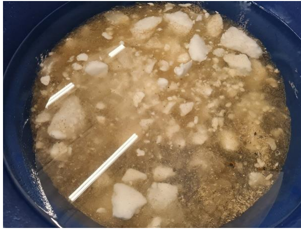
Figure 50. C&DW container with sodium sulfate solution.
